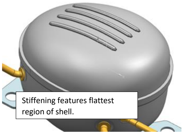
Figure 15-Rib Stiffened Outer Shell.
