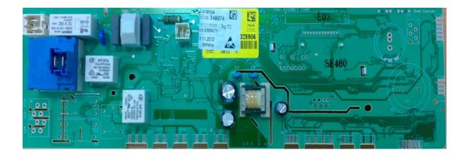
Remuved connector ( for ionizer and steam generator) from the main board. - different ionizer connection. New situation
