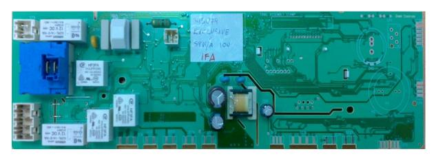
Control unit after changes - removed connector for ionizer and steam generator.
