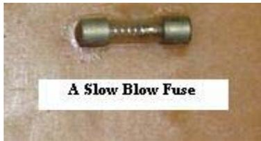
There are two basic types of fuses which is the fast acting and slow blow type. The fast acting fuse will open very quickly when their particular current rating is exceeded. This is very important for analogue multimeter, which can quickly be destroyed when too much current flows through them, for even a very small amount of time.
