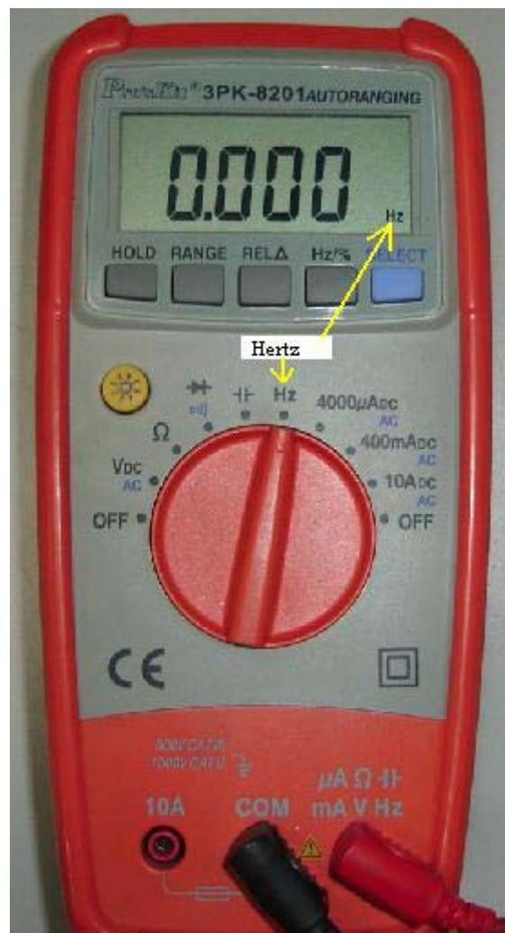
Frequency counter in a digital multimeter
