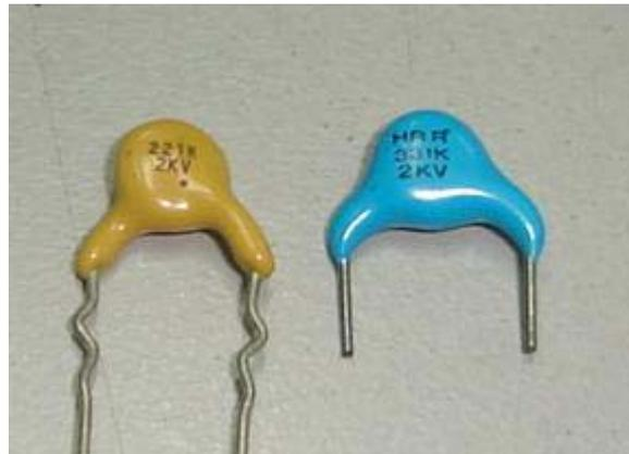
Resin coated ceramic disc capacitors
