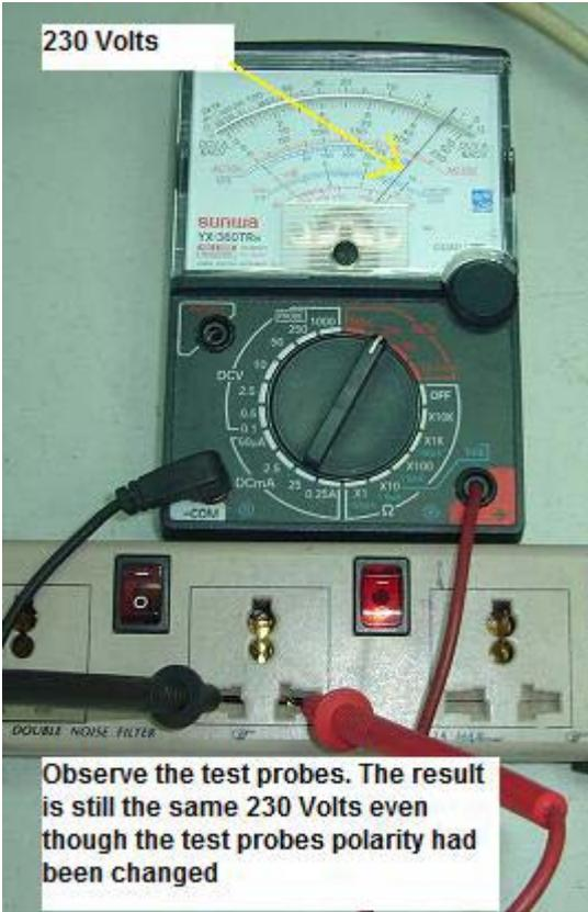
In order to accurately test AC and DC voltage, I only use the digital meter as it shows more precise reading than the analogue meter. Set your multimeter to its appropriate function (DCV or ACV), then select the proper range. Note, an auto ranging digital meter will select its own range. Place your test leads across (in parallel with) the part under test as shown in all the photos below and read voltage directly from the panel meter.
