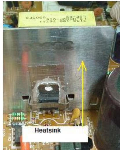
The heat generated by current flowing between the collector and emitter junctions of a transistor causes its temperature to rise. This heat must be conducted away from the transistor otherwise the temperature rise may be high enough to irreparably damage the P-N junctions inside the transistor. Power transistors produce a lot of heat, and are therefore usually mounted to a piece of aluminium with fins, called a heat sink.
