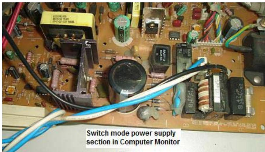
Switch Mode Power Transformer (SMPT) are used in switch mode power supplies in electronic equipment such as Computer Monitor, TV, DVD and etc. The function of SMPT is to convert the AC wave to some other value, lower or higher. The input is called primary winding while the outputs are secondary windings.
