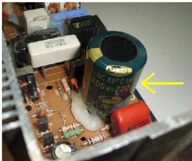
The large filter capacitor in power supply section
