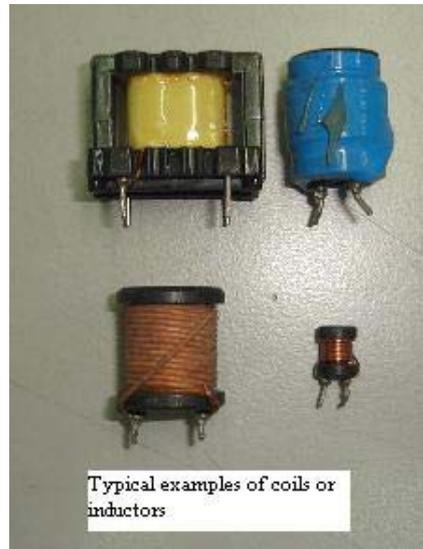
Testing coil is very easy compares to checking three leads components such as SCR, FET and etc. In general, a coil consists of many turns of wire wrapped around a common core. The core could be made of iron or even air. It is label as “L” on circuit board.
