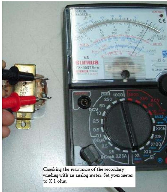
With power off, remove the transformer from the board and perform a resistance or continuity test on primary and secondary winding as shown on the picture of transformer below. If there is no resistance or ohms reading on the primary and secondary winding measured, suspect an open winding and the transformer need to be replaced. The advantage of this method is you are safe because no power is applied to the transformer.
