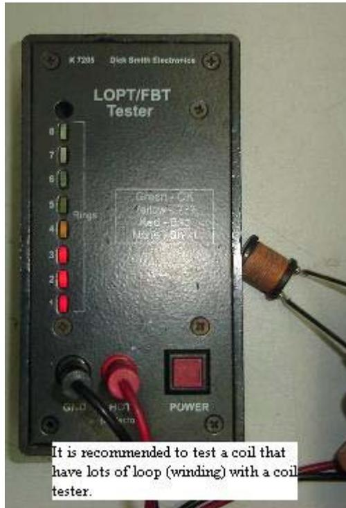
Now is the time to share my true case example- a computer dealer send me a monitor for repair with power blink symptom. Usually I do not straight away repair the monitor but I would first use the flyback tester to scan all the major coils (switch mode transformer, flyback transformer, B+ coil and horizontal deflection coil) before using my digital or analogue meter to do testing.
