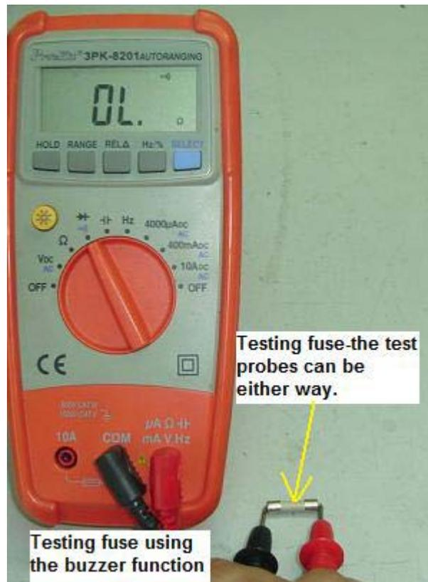
The red and black test probes can be either way when test on fuses
