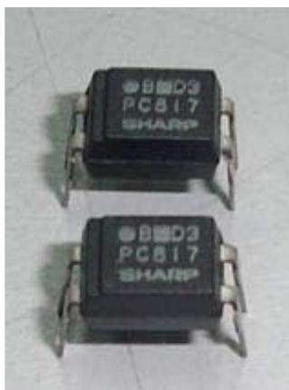
Many technicians and engineers do not know that they can actually test the optocoupler with their analogue multimeter. Most of them thought that there is no way of **testing** an IC with an analogue meter. Since we already knew the optocoupler pin out from the schematic diagram, testing this IC is just the same as measuring a normal bipolar transistor and LED.
